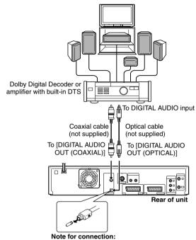
Remove the protection cap from the optical cable.
